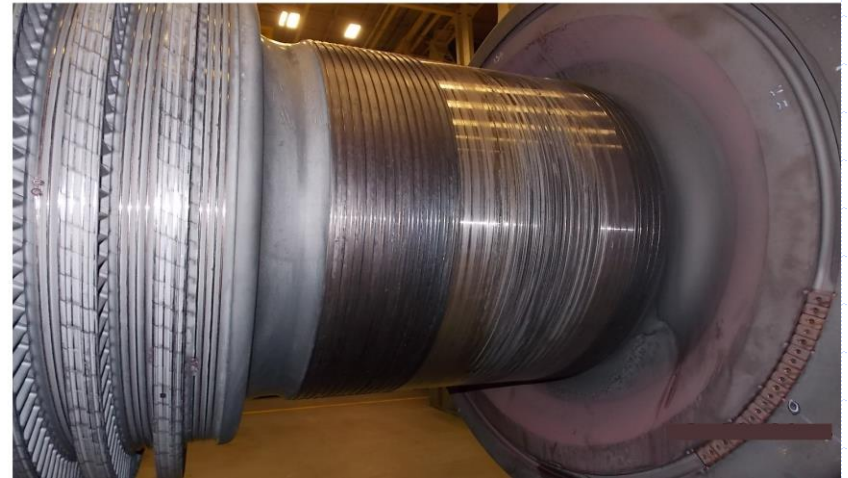
Vibration Alarm Not Armed – Rub Not Detected - Resulted in Bowed Rotor
